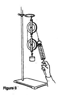
5. Set up a block and tackle with a double fixed and a double movable pulley. See the example on the front desk to help you set this up.
